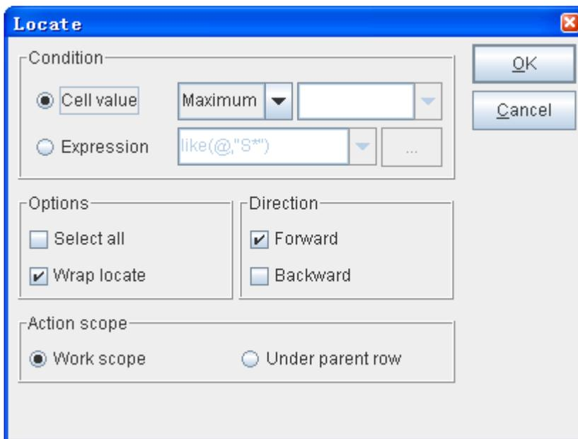
Select the locating condition of **Maximum** cell value. After locating, the cursor will move to the cell C3.
